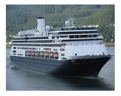
**Built:** 1999 Category: 4-stars GT: 61214 tonnes Shipyard: Fincantieri Length: 237.7m 32.20m Beam: Draught: 5.15m Total output: 43200 kW Speed: 23 knots Stabilisers: Yes Passenger decks: 10 Passengers: 1432 Crew: 615 Tender (150 seats): 6 **Hospital:** Yes Agent: Inchcape: Ph: 40515211 **Ship's Registry:** The Netherlands Owner: Carnival Corporation & plc **Operator:** Holland America Line
